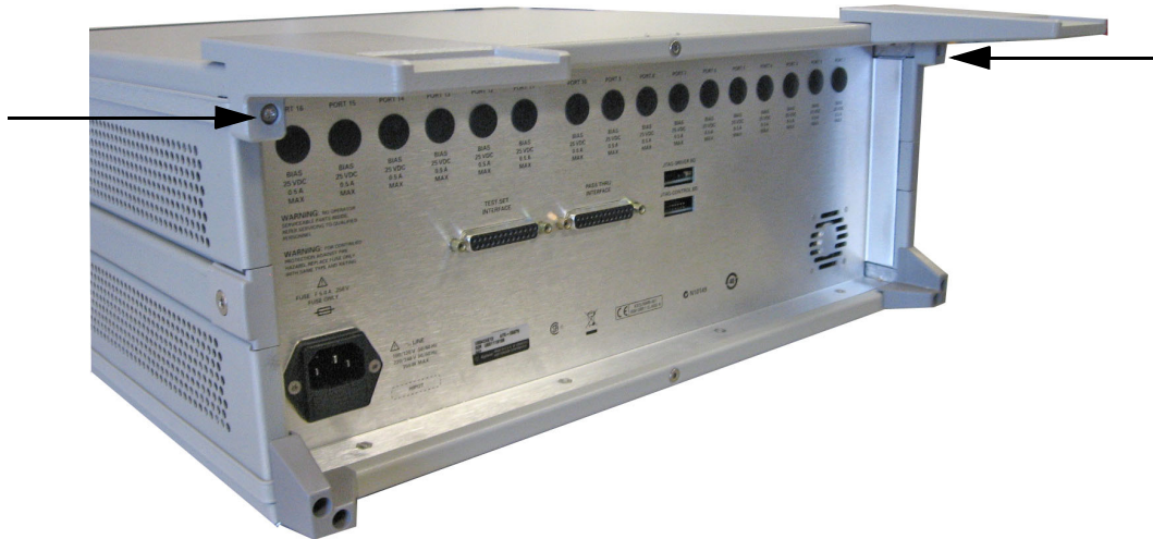
Figure 8 Install Locking Feet on U3022AH10
