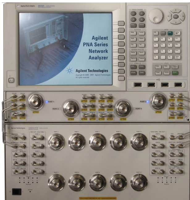
Figure 2 N5242A 4-Port PNA-X with Test Set
