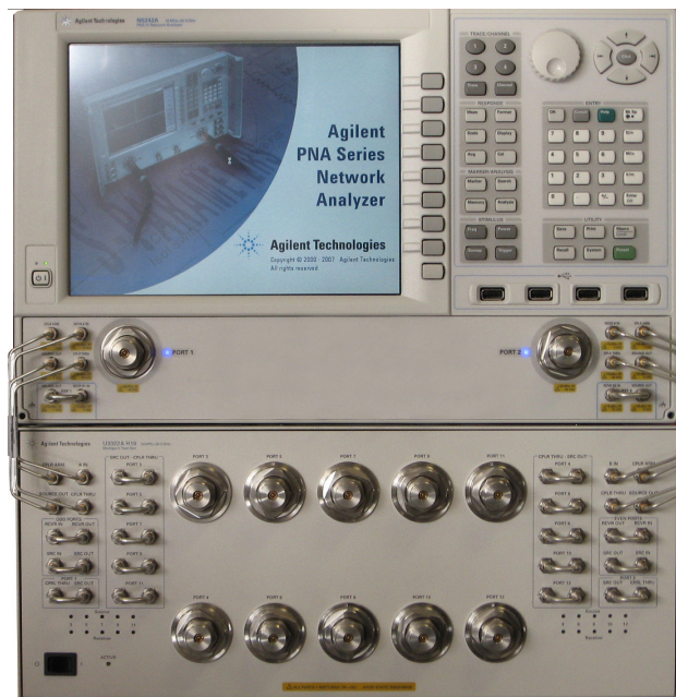
Figure 1 N5242A 2-Port PNA-X with Test Set
